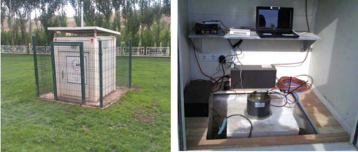
Figure 6. Internal and External Appearance of a TR-NSMN Station.
