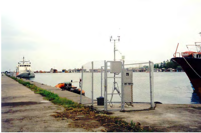
Figure-3.7: Trabzon digital and automatic tide gauge
